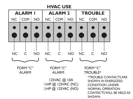
In the event of a fire alarm, certain equipment may be required to be shut down. For example, shut down may be achieved by interrupting the fan supply source to that particular piece of equipment when wired as indicated (shown below).
